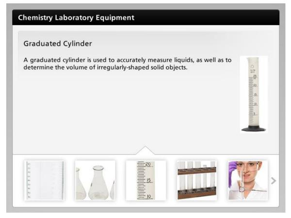
A graduated cylinder is used to accurately measure liquids, as well as to determine the volume of irregularly-shaped solid objects.
