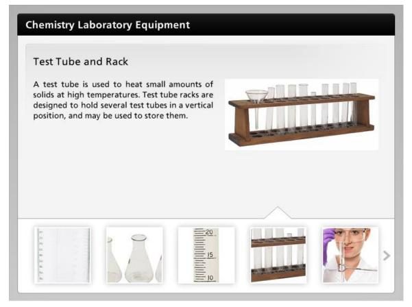
A test tube is used to heat small amounts of solids at high temperatures. Test tube racks are designed to hold several test tubes in a vertical position, and may be used to store them.
