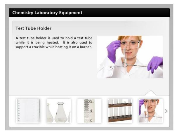
A test tube holder is used to hold a test tube while it is being heated. It is also used to support a crucible while heating it on a burner.
