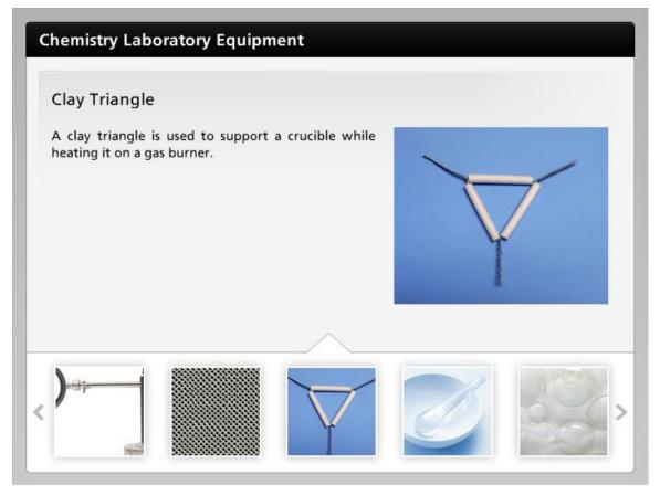
A clay triangle is used to support a crucible while heating it on a gas burner.
