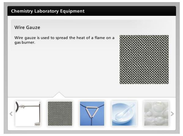
Wire gauze is used to spread the heat of a flame on a gas burner.
