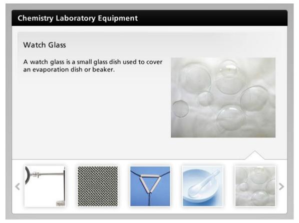
A watch glass is a small glass dish used to cover an evaporation dish or beaker.
