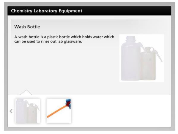
A wash bottle is a plastic bottle which holds water which can be used to rinse out lab glassware.
