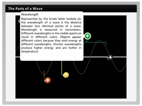
Represented by the Greek letter lambda  $(\lambda)$ , the wavelength of a wave is the distance between two identical points of a wave. Wavelength is measured in nanometers. Different wavelengths in the visible spectrum result in different colors. Objects appear different colors because they emit energy at different wavelengths. Shorter wavelengths produce higher energy and are hotter in temperature.
