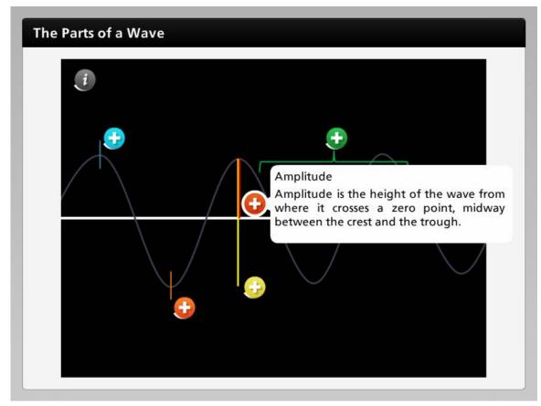
Amplitude is the height of the wave from where it crosses a zero point, midway between the crest and the trough.
