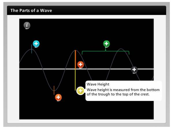
Wave height is measured from the bottom of the trough to the top of the crest.
