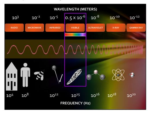
The electromagnetic spectrum starts with very long radio waves. These waves have a wavelength of 102 meters and a frequency of 300 kHz. The electromagnetic spectrum includes radio waves, microwaves, infrared, visible light, ultraviolet, x-rays, and gamma rays. According to the wave model, visible light consists of a small portion of the electromagnetic spectrum.
