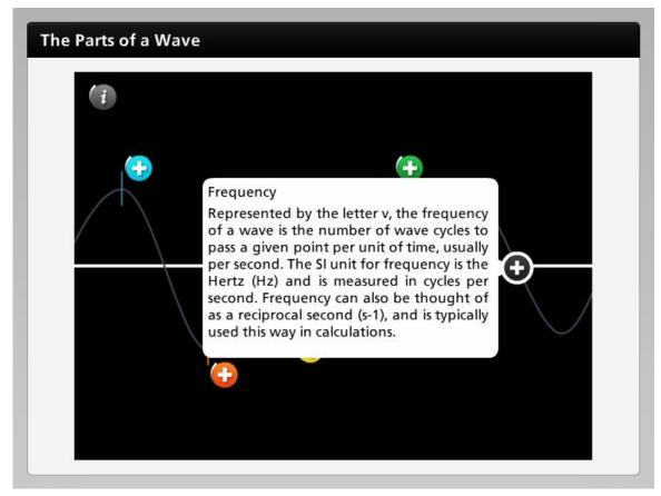
Represented by the letter v, the frequency of a wave is the number of wave cycles to pass a given point per unit of time, usually per second. The SI unit for frequency is the Hertz (Hz) and is measured in cycles per second. Frequency can also be thought of as a reciprocal second (s-1), and is typically used this way in calculations.
