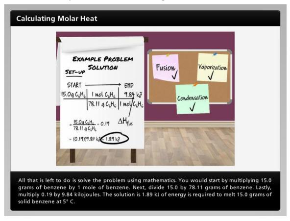
All that is left to do is solve the problem using mathematics. You would start by multiplying 15.0 grams of benzene by 1 mole of benzene. Next, divide 15.0 by 78.11 grams of benzene. Lastly, multiply 0.19 by 9.84 kilojoules. The solution is 1.89 kJ of energy is required to melt 15.0 grams of solid benzene at  $5^{\circ}$  C.
