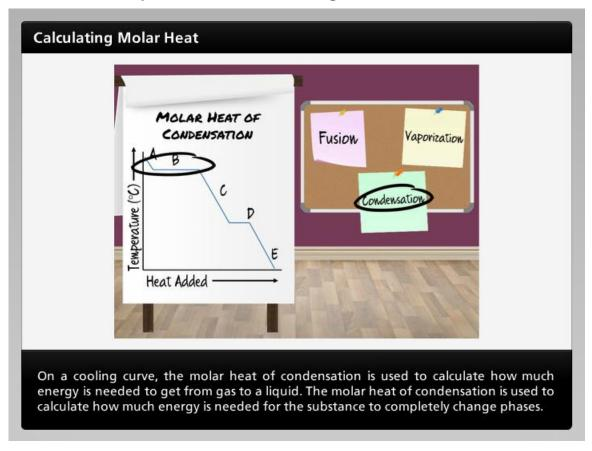
On a cooling curve, the molar heat of condensation is used to calculate how much energy is needed to get from gas to a liquid. The molar heat of condensation is used to calculate how much energy is needed for the substance to completely change phases.
