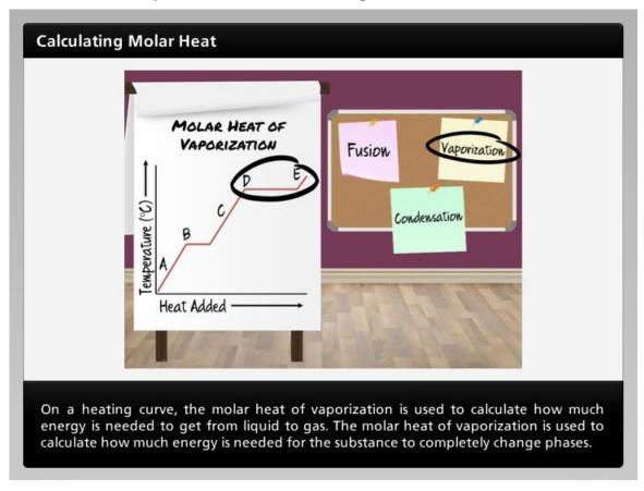
On a heating curve, the molar heat of vaporization is used to calculate how much energy is needed to get from liquid to gas. The molar heat of vaporization is used to calculate how much energy is needed for the substance to completely change phases.
