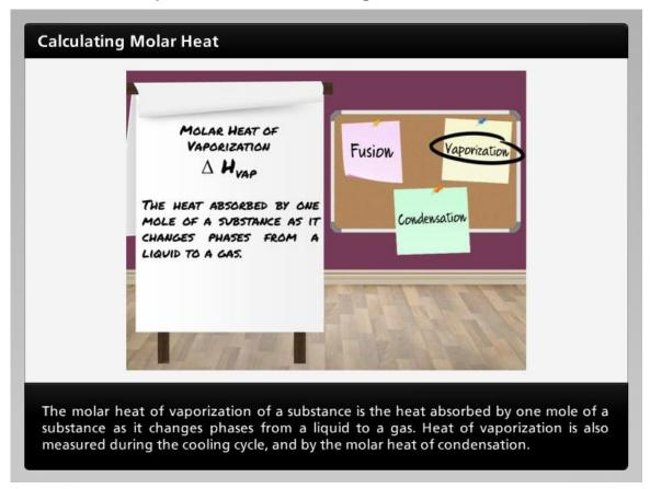
The molar heat of vaporization of a substance is the heat absorbed by one mole of a substance as it changes phases from a liquid to a gas. Heat of vaporization is also measured during the cooling cycle, and by the molar heat of condensation.
