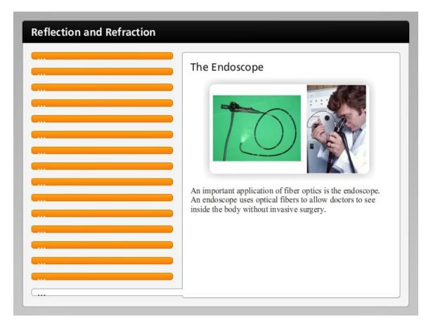
An important application of fiber optics is the endoscope. An endoscope uses optical fibers to allow doctors to see inside the body without invasive surgery.
