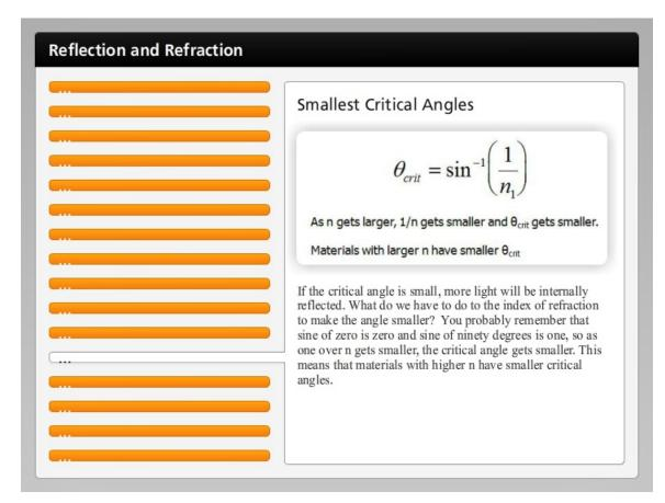
If the critical angle is small, more light will be internally reflected. What do we have to do to the index of refraction to make the angle smaller? You probably remember that sine of zero is zero and sine of ninety degrees is one, so as one over n gets smaller, the critical angle gets smaller. This means that materials with higher n have smaller critical angles.
