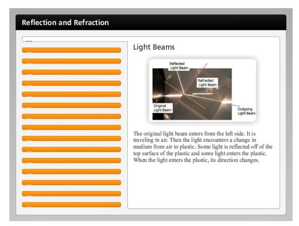
The original light beam enters from the left side. It is traveling in air. Then the light encounters a change in medium from air to plastic. Some light is reflected off of the top surface of the plastic and some light enters the plastic. When the light enters the plastic, its direction changes.
