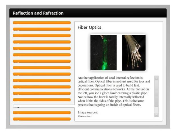
Another application of total internal reflection is optical fiber. Optical fiber is not just used for toys and decorations. Optical fiber is used to build fast, efficient communications networks. At the picture on the left, you see a green laser entering a plastic pipe. Notice how the laser is totally internally reflected when it hits the sides of the pipe. This is the same process that is going on inside of optical fibers.
