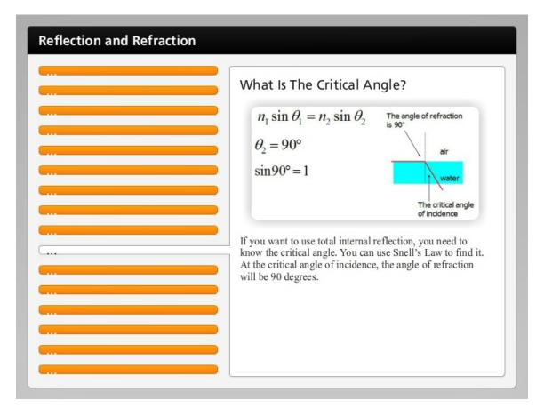
If you want to use total internal reflection, you need to know the critical angle. You can use Snell's Law to find it. At the critical angle of incidence, the angle of refraction will be 90 degrees.
