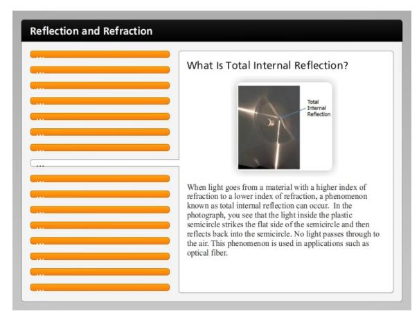
When light goes from a material with a higher index of refraction to a lower index of refraction, a phenomenon known as total internal reflection can occur. In the photograph, you see that the light inside the plastic semicircle strikes the flat side of the semicircle and then reflects back into the semicircle. No light passes through to the air. This phenomenon is used in applications such as optical fiber.
