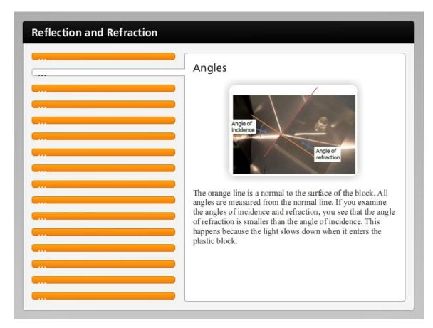
The orange line is a normal to the surface of the block. All angles are measured from the normal line. If you examine the angles of incidence and refraction, you see that the angle of refraction is smaller than the angle of incidence. This happens because the light slows down when it enters the plastic block.
