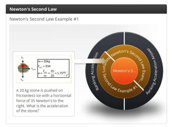
First, it will be helpful to draw a free body diagram of the stone. We've got the gravitational force pulling down on the stone, the normal force from the ice pushing back perpendicular to the surface, and the push force of thirty five Newton's to the right.
