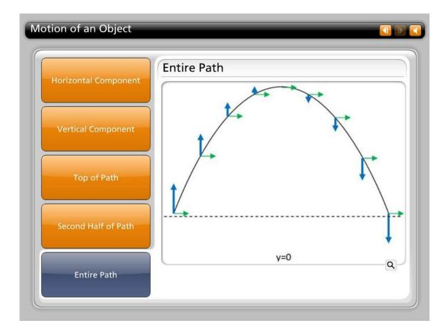
Now look at the entire path of the object. How does the initial height compare to the final height? Since the object returns to the same height from which it began, the total vertical displacement will be zero from the beginning to the end of the flight,. We'd write that in an equation as y equals zero. We'll apply each of these phenomena as we look at several examples of projectile motion.
