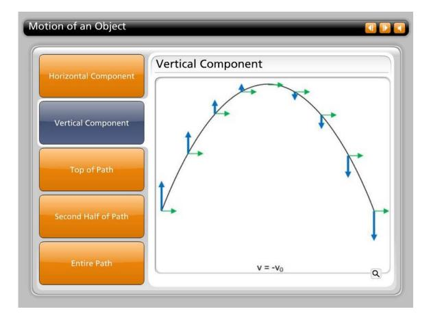
Look at what happens to the blue arrows over the entire flight. The vertical component of the velocity begins positive, but you can see that the length of the arrows initially decreases due to the downward acceleration of gravity. Later, the arrows get longer, but they are pointing downwards, indicating that the vertical component of the velocity is now in a negative direction as the object continues to accelerate downwards due to gravity.
