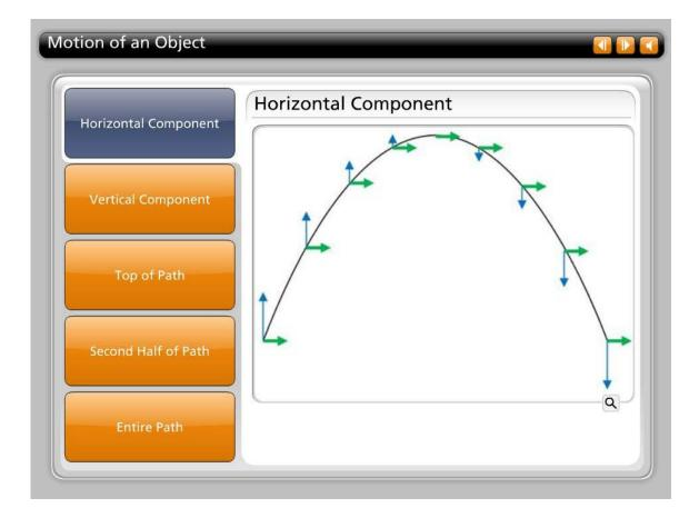
What do you notice about the green arrows? Do you see how they are all the same length? This indicates that the horizontal component of the velocity is constant. Since there is no acceleration in the horizontal direction, the horizontal component of the velocity does not change.
