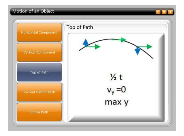
What happens to the blue arrows at the top of the path? You should notice that the vertical component of velocity reaches zero at the highest point of motion. You should recall this from the lesson on freefall.
