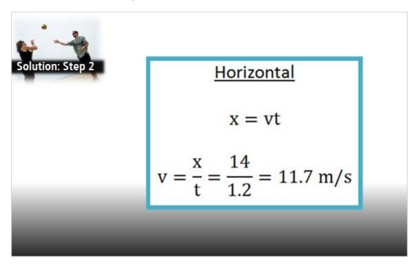
The horizontal velocity is fairly straightforward. We know that the displacement is the velocity times time, so the velocity is displacement divided by time. Substituting and solving, we see that the initial horizontal velocity is eleven point seven meters per second.
