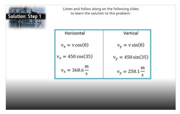
Again, the best way to start any projectile motion problem is to identify the horizontal and vertical variables. We don't know the time or the displacement in the horizontal direction, but we can determine the horizontal component of the velocity.
