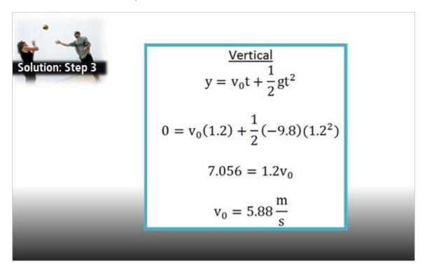
In the vertical direction, to solve for the initial velocity, we can use the equation y equals v zero t plus one half g t squared.
