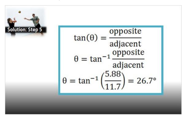
Now, to determine the angle, we need to use an inverse trig function. The tangent of the angle is the opposite over the adjacent, so the angle is equal to the inverse tangent of the opposite over the adjacent.
