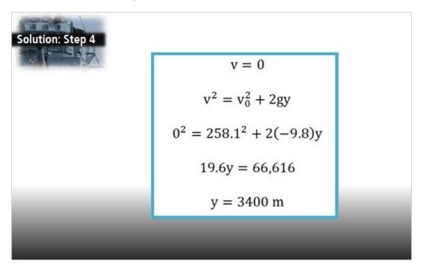
Since we know the initial vertical velocity, we can find the maximum height by recognizing that this is where the vertical velocity momentarily slows to zero.
