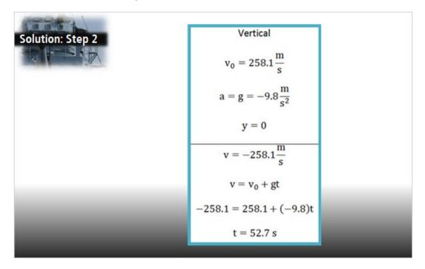
The y component of the initial velocity is the initial y velocity. Also in the vertical direction, we know the gravitational acceleration of nine point eight meters per second squared in a negative direction. The vertical displacement is zero since the shell rises and falls back to its initial height.
