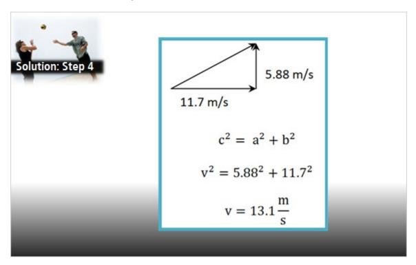
Now, we need to combine these initial horizontal and vertical components of the velocity. To do this, we will line them up head to tail to form a right triangle and use the Pythagorean Theorem to determine the hypotenuse, which is the magnitude of the initial velocity.
