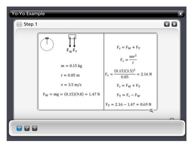
Since understanding the forces is so critical, your first step is to draw a free body diagram of the yo-yo. You see that there are two forces acting on the yo-yo while it is at the top of its path: The gravitational force and the tension force. Both forces are pointing down, which is towards the center of the circular path.
