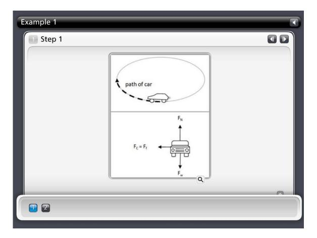
First, you must draw a free body diagram of the car. It is easiest to see the forces if we see the car coming towards us. There is the gravitational force directed straight down, and the normal force directed straight up. There must be an additional force pointed towards the center of the circle, left in this case, which provides the centripetal force necessary to complete the turn. In this case, it is the static friction of the tires on the road that provide this force.
