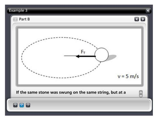
In the previous problem, when the stone was swung at fifteen meters per second, there was a tension of one hundred fifty Newtons. If the same stone was swung on the same string, but at a velocity of only five meters per second, what would be the tension in the string?
