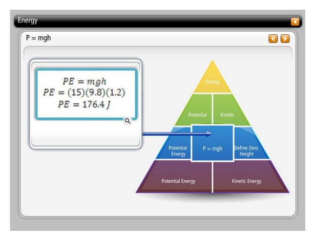
Again, if the box is fifteen kilograms, and it is lifted to a shelf that is one point five meters above the floor, you'd calculate the potential energy with the equation PE equals mg h. Substituting and solving, you find the potential energy on the shelf to equal one hundred seventy six point four Joules. This is the same amount you calculated earlier using Work.
