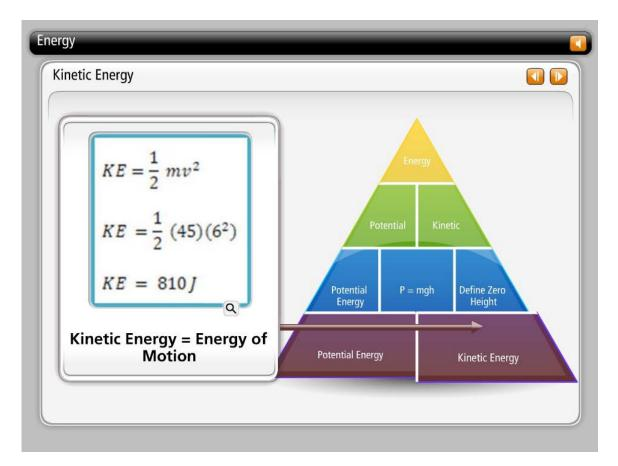
Kinetic energy is the energy of motion. When an object is moving it has kinetic energy. When you do work on an object and it speeds up, the object has gained kinetic energy.
