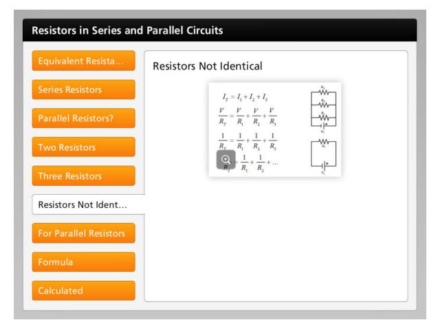
But what if the resistors are not identical? How can you find the equivalent resistance for parallel resistors that have different values? You need an equation to do this.
