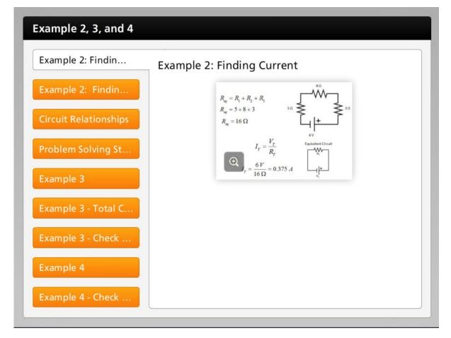
In this circuit, a six volt battery is used with a five ohm, eight ohm and 3 ohm resistors. What is the equivalent resistance? What is the current delivered by the battery?
