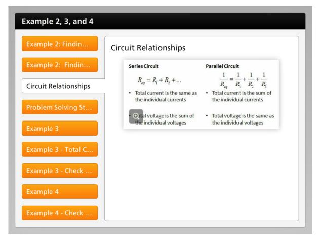
In this lesson you learned how to determine the effect of connecting resistors in series or parallel on the total resistance of the circuit. Remember that total does not mean to add values, it refers to the combined effect of all of the resistors in a circuit. Equivalent resistance is the value of a single resistor that could replace a combination of resistors.
