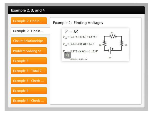
Since all the elements are in series, they all have the same current of zero point three seven five amps. What is the voltage drop across each resistor?
