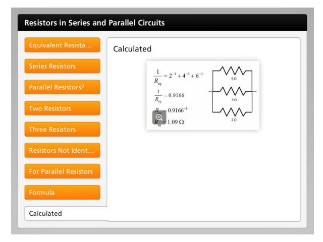
Enter in your calculator two to the negative one plus four to the negative one plus six to the negative one.
