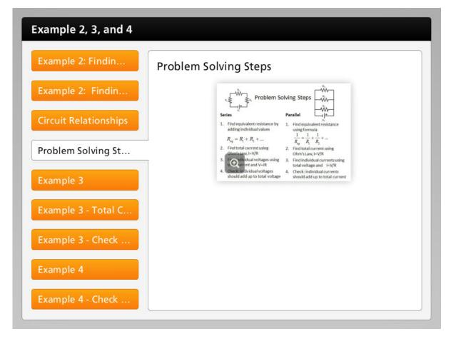
Knowing the relationships between voltage, current and resistance for series and parallel arrangements will help you in problem solving. There are two basic types of problems in this topic: series circuits and parallel circuits.
