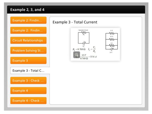
Now that you have found the total resistance, use Ohm's Law to find the total current. The insect sees the vulture over the rabbit, so I equals V over R. Substituting the values for total resistance and total voltage, we see the total current is fifteen point six amps.
