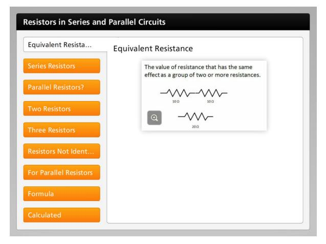
It will be easier to analyze circuits when you simplify complicate arrangements of resistors. To do this, you will use equivalent resistance. The equivalent resistance is a value of resistance that has the same effect as a group of two or more resistances.
