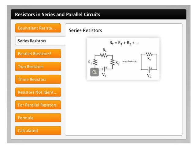
You can replace two or more series resistors in a circuit with one resistor that has a resistance equal to the sum of the individual resistances. In the equation, the ellipses are uses to remind you that you can include as many terms as you have resistors in series.
