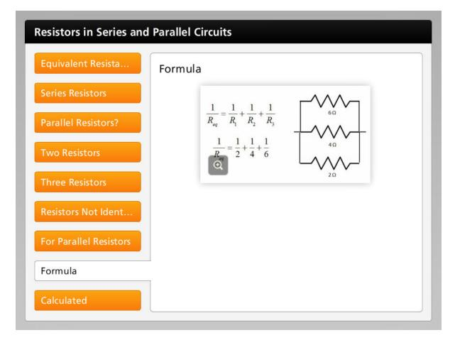
Let's try an example to illustrate how this formula is used. If the three resistors are two ohms, four ohms and six ohms, let's find the equivalent resistance.
