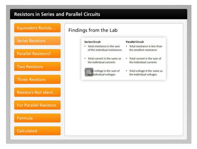
In the lab you found the total resistance of each circuit experimentally by using Ohm's Law, R equals V over I. When you compared this total resistance to the individual values, you should have noted differences between the series and parallel circuits. Note that the word total is used to refer to the value for the entire circuit. Those differences are summarized here.
