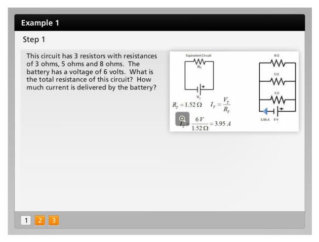
This circuit has three resistors with resistances of three ohms, five ohms and 8 ohms. The battery has a voltage of six volts. What is the total resistance of this circuit? How much current is delivered by the battery?
