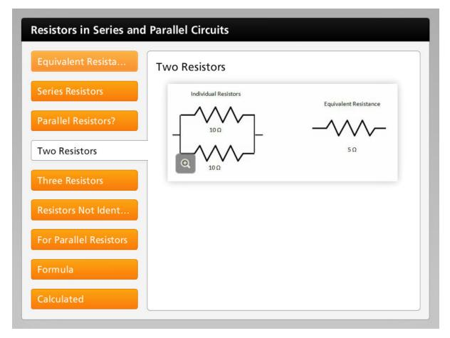
If two ten ohm resistors in are put in parallel, this is equivalent to one five ohm resistor. The area for current flow has been doubled, which cuts the resistance in half.
