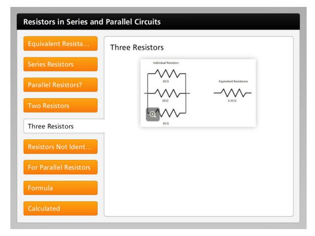
If the three ten ohm resistors in are put in parallel, this is equivalent to one three point three ohm resistor. The area for current flow has been tripled, which cuts the resistance to one-third of its original value.
