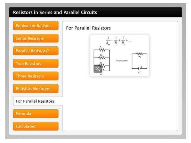
To find the equivalent resistance for parallel resistors you add the reciprocals of the resistances. This sum is the reciprocal of the equivalent resistance. Let's try an example to see how this works out.
