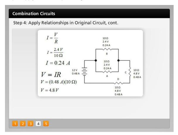
Now you can use Ohm's Law to find the current through resistors A and B. I equals V over R. Substituting values, we see that the current is zero point two four amps. You probably noticed that half of the current is going through each of the parallel branches. This happens because the two branches have equal resistances. If the resistances were different, the currents would be different also. However, the voltage of parallel branches are always the same even if the resistances are different.
