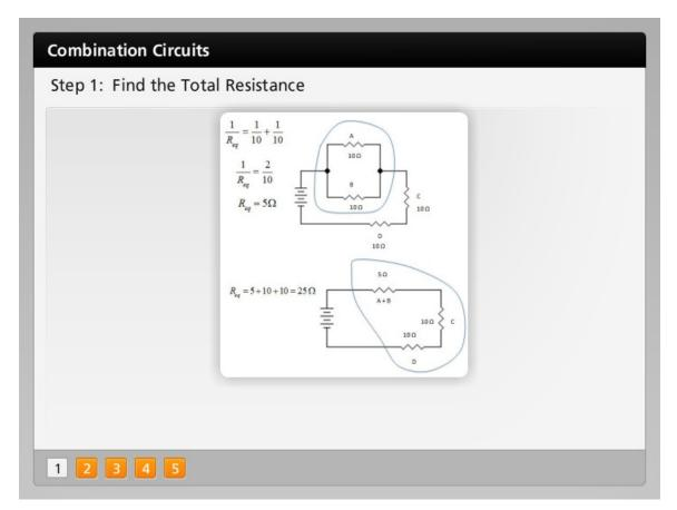
To illustrate this process, let's look at an example. In this example circuit, four identical resistors, each with a resistance of ten ohms, are connected to a battery with a potential difference of twelve volts.
