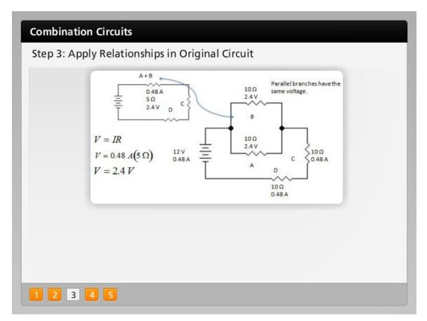
Go back to the original diagram. You now know how much current is leaving the battery, zero point four eight amps. Resistors C and D are in series with the battery, so they have the same current as the battery.
