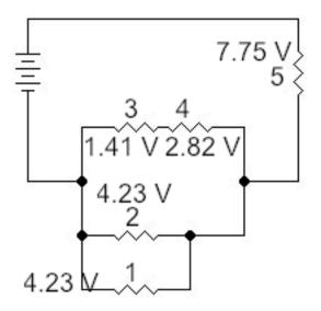
Kirchoff's Loop Rule states that when you go around a circuit the sum of the voltage drops must equal the voltage of the battery. There are three different paths. Resistor 5 + Resistor 1; 7.75 + 4.23 = 11.98 pretty close to 12 V Resistor 5 + Resistor 2; 7.75 + 4.23 = 11.98 Resistor 5 + Resistor 3 + Resistor 4; 7.75 + 1.41 + 2.82 = 11.98
