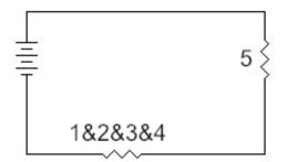
• Combine this result with 5 in series.  $2.73 + 5 = 7.73 \Omega$ ; this is the total resistance Battery Current (Using Ohm's Law):
