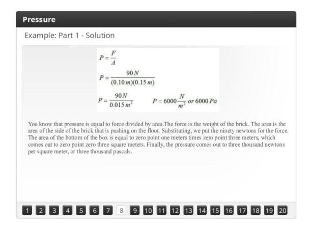
You know that pressure is equal to force divided by area. The force is the weight of the brick. The area is the area of the side of the brick that is pushing on the floor. Substituting, we put the ninety newtons for the force. The area of the bottom of the box is equal to zero point one meters times zero point three meters, which comes out to zero point zero three square meters. Finally, the pressure comes out to three thousand newtons per square meter, or three thousand pascals.
