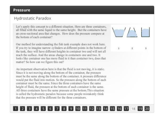
Let's apply this concept to a different situation. Here are three containers, all filled with the same liquid to the same height. But the containers have an cross-sectional area that changes. How does the pressure compare at the bottom of each container?
