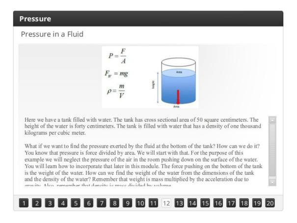
Here we have a tank filled with water. The tank has cross sectional area of 50 square centimeters. The height of the water is forty centimeters. The tank is filled with water that has a density of one thousand kilograms per cubic meter.
