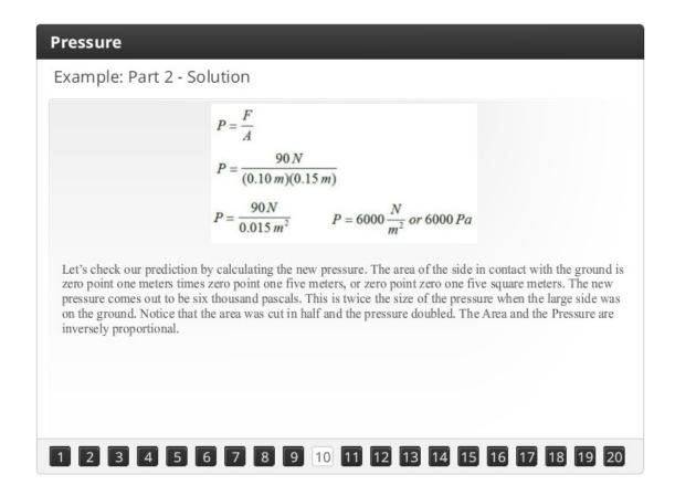
Let's check our prediction by calculating the new pressure. The area of the side in contact with the ground is zero point one meters times zero point one five meters, or zero point zero one five square meters. The new pressure comes out to be six thousand pascals. This is twice the size of the pressure when the large side was on the ground. Notice that the area was cut in half and the pressure doubled. The Area and the Pressure are inversely proportional.
