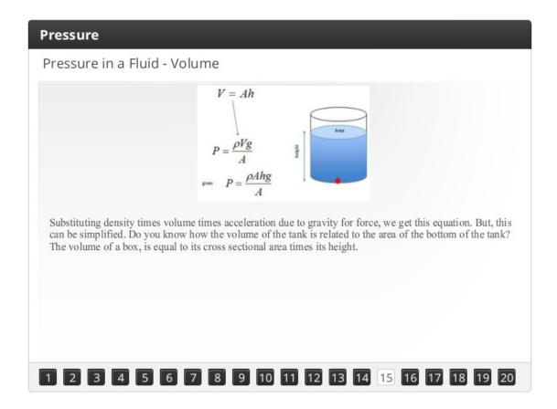
Substituting density times volume times acceleration due to gravity for force, we get this equation. But, this can be simplified. Do you know how the volume of the tank is related to the area of the bottom of the tank? The volume of a box, is equal to its cross sectional area times its height.
